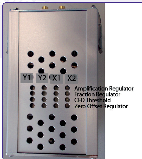
Figure 13: Labeling of discriminator threshold and amplification regulators.
